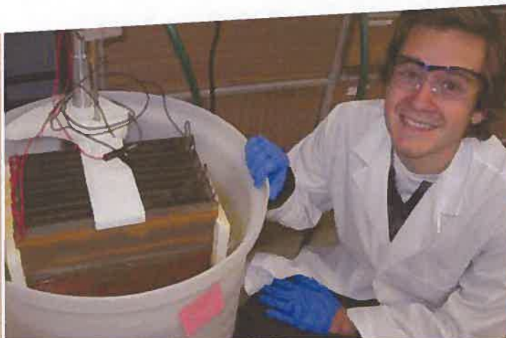
Engineering graduate student Case van Genuchten with an Electro-chemical Arsenic Removal (ECAR) prototype device for removing arsenic from drinking water in Bangladesh.
